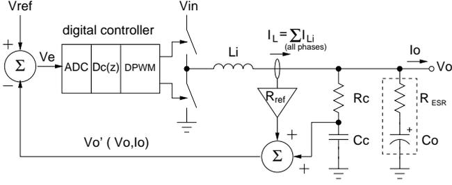
Fig. 5. Implementation of optimal voltage positioning with a digital controller.
