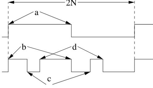
Fig. 10. Possible oscillation modes of the ring. The upper waveform is the fundamental sequence with the period of  $2N$ , where “a” denotes the only pair of edges. The lower waveform is a sequence of 3 pairs of edges with the same period, where “b”, “c” and “d” denote the 3 pairs of edges.
