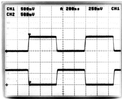
Fig. 12. Differential output of one ring oscillator delay stage. The upper waveform is taken from one tap on one stage of the ring, and the lower waveform is taken from the symmetric tap from the same stage. The vertical scale is  $500\text{mV}/\text{div}$ , and horizontal scale is  $200\text{ns}/\text{div}$ .
