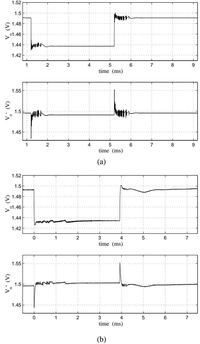
Fig. 6. Transient response of a prototype digitally controlled multi-phase buck converter with parameters from Table II, resulting from a 10A load current step: (a) simulation, and (b) experimental results.  $V_o$  is the output voltage, and  $V_o'$  is the quantity compared to  $V_{ref}$  to form the error signal.
