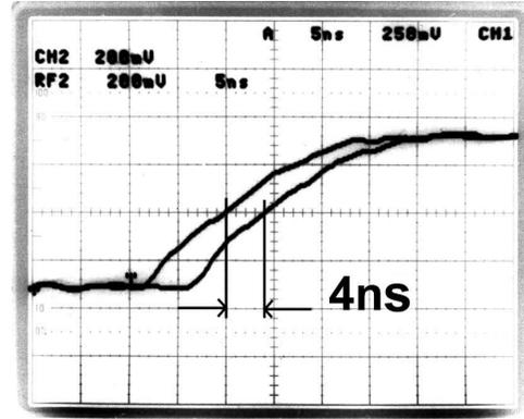
Fig. 13. 8-Bit resolution is achieved between two adjacent outputs of a ring oscillator delay cell. At  $1\text{MHz}$  oscillation frequency, the resolution is  $4\text{ns}$ .
