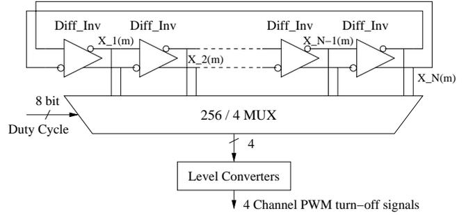
Fig. 8. PWM generation block diagram
