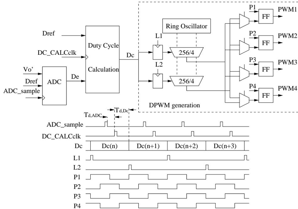
Fig. 14. Block diagram and timing of proposed digital controller IC
