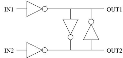
Fig. 9. Ring oscillator delay cell
