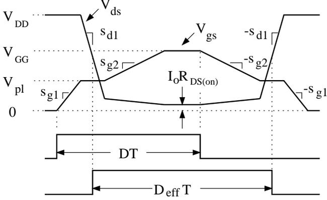
Fig. 3. Duty cycle variation due to the MOSFET switching characteristic.
