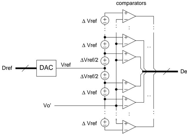
Fig. 7. Block diagram of a windowed ADC. It implements both an ADC and an error amplifier.
