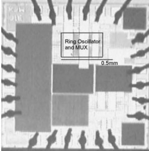
Fig. 11. Die photo of ring-oscillator-MUX test chip in  $0.25\mu\text{m}$  CMOS process
