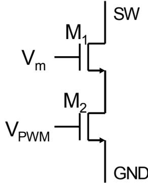
Figure 4.10: Cascode structure for low side switch.
