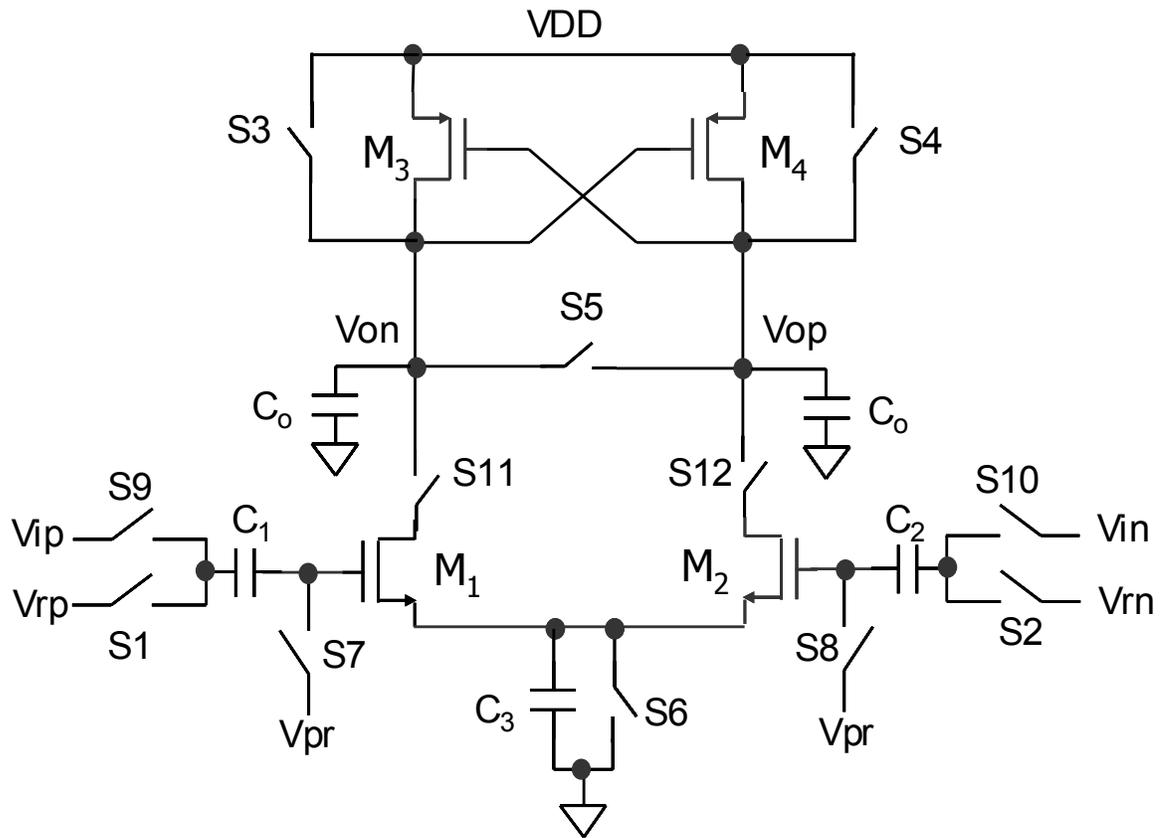
Figure 4.6: Schematic of the differential zero-DC-current comparator.
