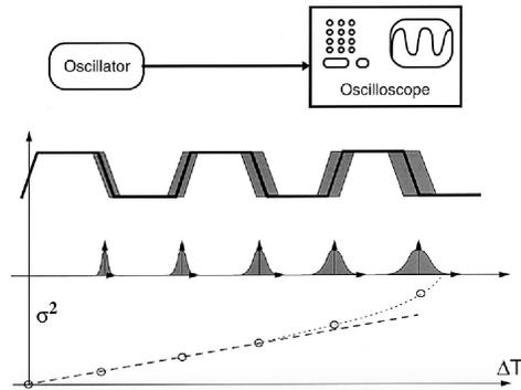
Figure 7.4: Clock jitter increasing with time [3]
