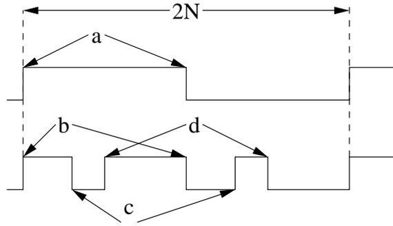
Figure 7.2: Possible oscillation patterns in a ring oscillator. The upper waveform is the fundamental pattern with the period of  $2N$ , where “a” denotes the one pair of transition edge. The lower waveform is a pattern with 3 pairs of transition edges, where “b”, “c” and “d” denote the three pairs of edges.
