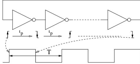
Figure 7.1: Single-ended ring oscillator with fundamental oscillation mode
