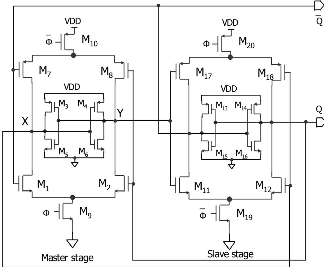
Figure 6.2: Schematic of proposed master-slave T flip-flop.
