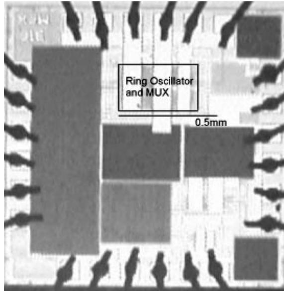
Figure 6.5: Die photo of an 8-bit ring-MUX DPWM test chip in 0.25- $\mu\text{m}$  CMOS process.
