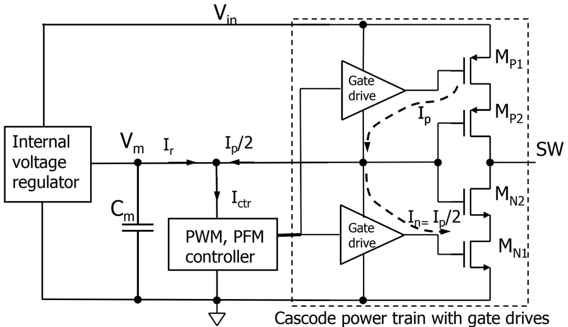
Figure 4.11: Block diagram of internal power management
