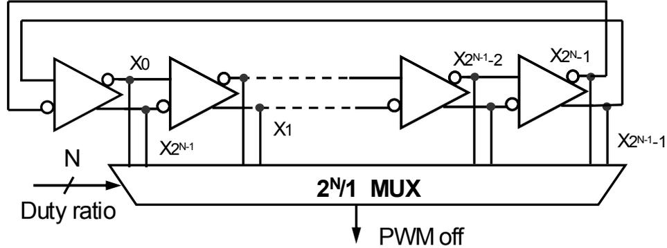
Figure 6.4: Block diagram of an N-bit ring-MUX DPWM.
