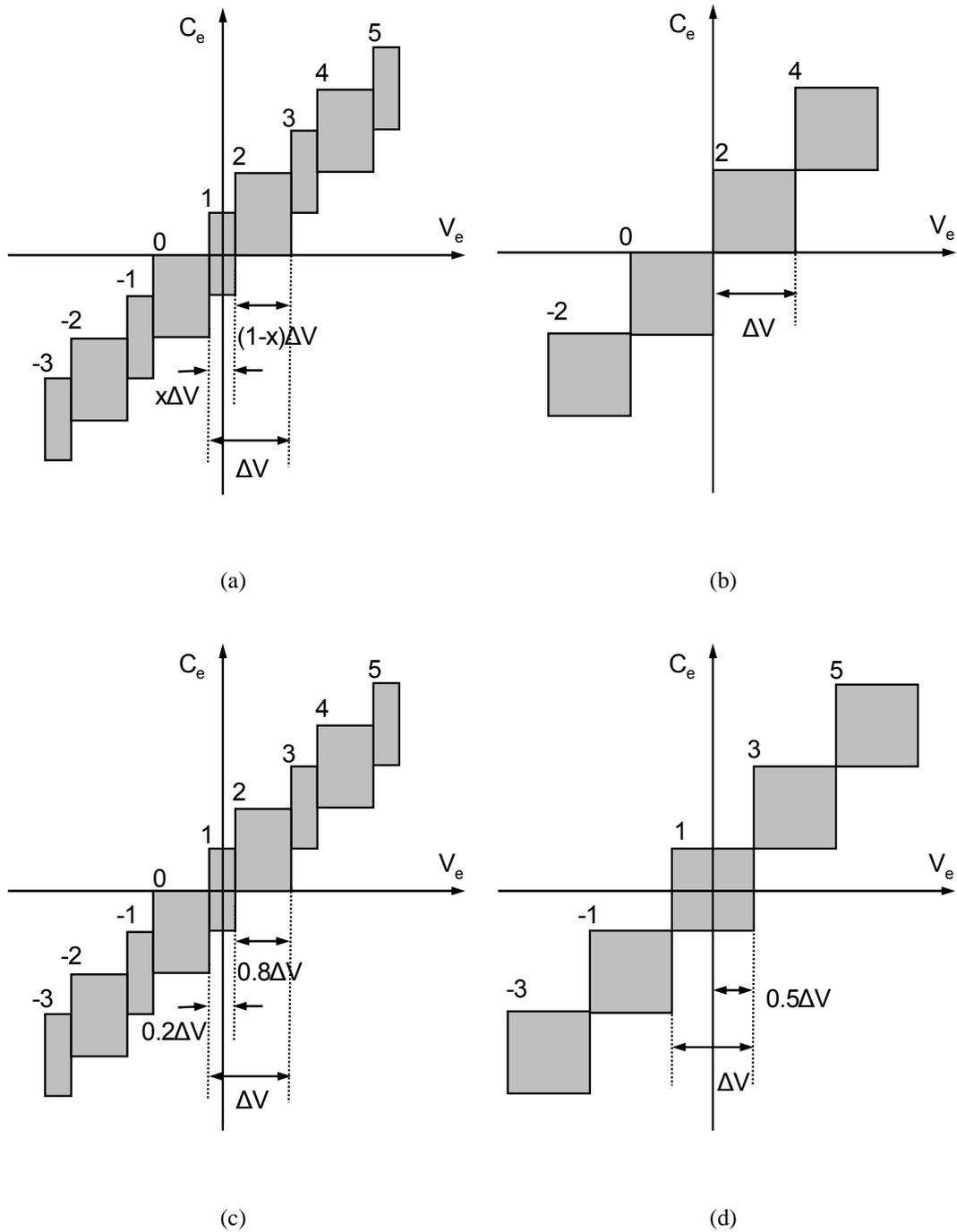
Figure 5.4: Uncertainty range of output code  $C_e$  (a) general form with  $f_0 = (n + x)f_s$ , where  $n$  is an integer and  $x \in [0, 1)$ , and three special case with (b)  $x=0$ , (c)  $x=0.1$ , (d)  $x=0.5$ , respectively.
