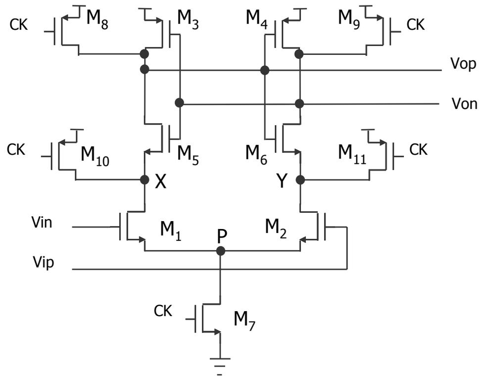
Figure 4.9: Schematic of zero-DC-biasing current comparator. [2]
