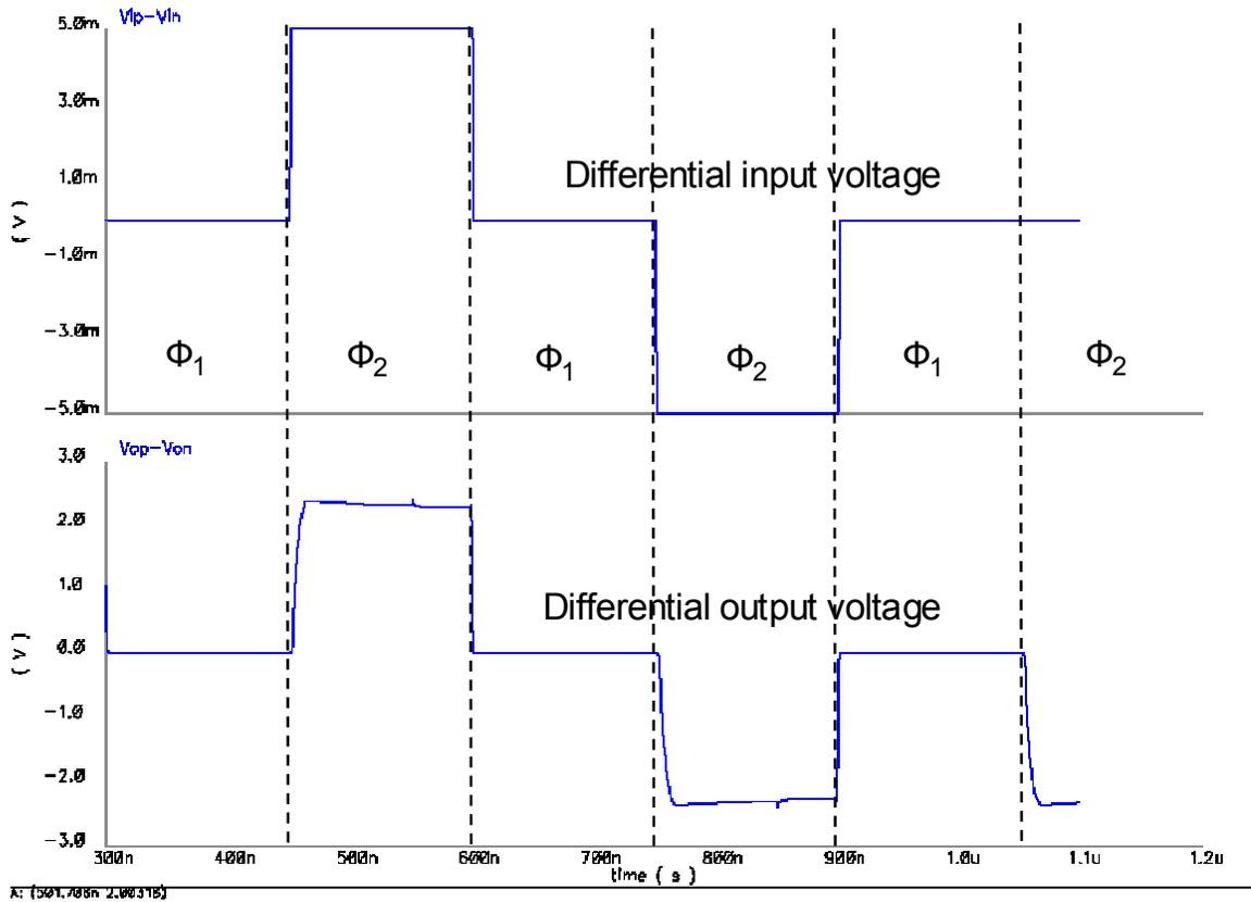
Figure 4.7: Simulated waveforms of the differential zero-DC-current comparator.
