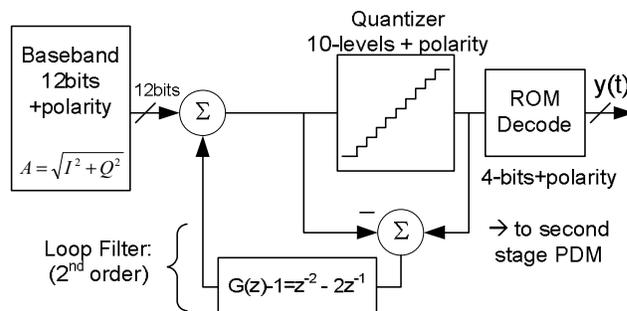
Fig. 4 Error-feedback digital  $\Delta\Sigma$  modulator
