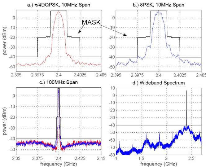
Fig. 11 Transmitter output spectrum, 100kHz RBW
