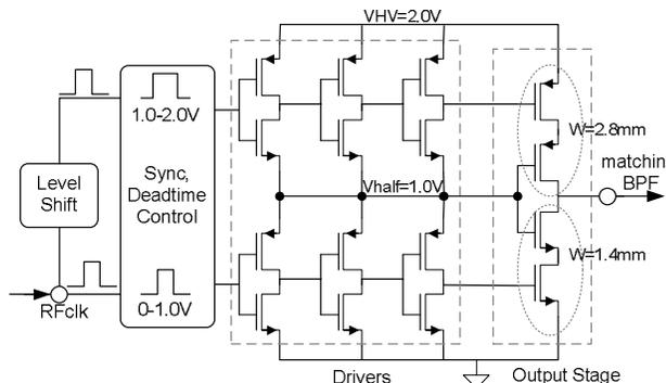
Fig. 2 CMOS Class-D cascode PA
