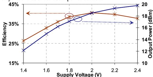
Fig. 8 Efficiency and output power vs supply voltage
