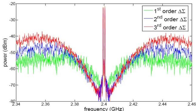
Fig. 5  $\Delta\Sigma$  Modulator: 1<sup>st</sup>, 2<sup>nd</sup>, 3<sup>rd</sup>-order comparison
