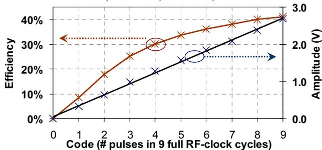
Fig. 9 Efficiency and linearity vs pulse-density
