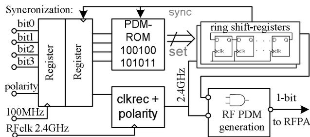
Fig. 6 Pulse-density modulator block
