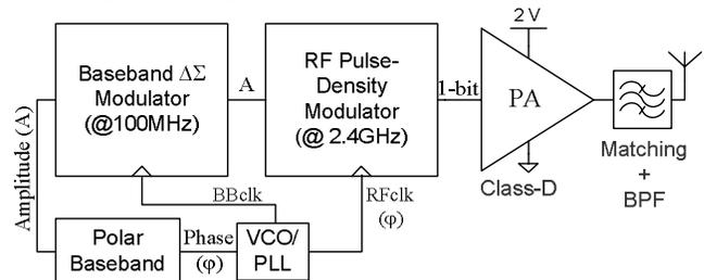
Fig. 1 Digital polar modulation architecture
