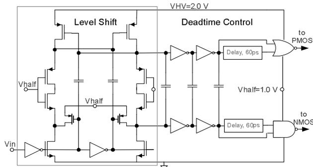
Fig. 3 Level shift and deadtime control
