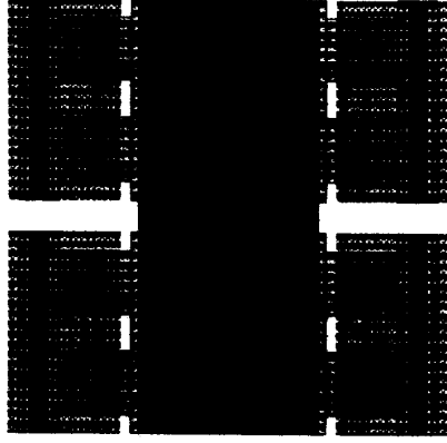
Figure 4: Layout of Fabricated Device. Top section is primary, bottom is secondary. Approximate dimensions of each plate (dark area) are 50\mu\text{m} ( w ) \times 30\mu\text{m} ( l ).
