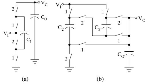
Fig. 4. Switch-level diagram of a) 1:2 converter, b) 3:2 converter
