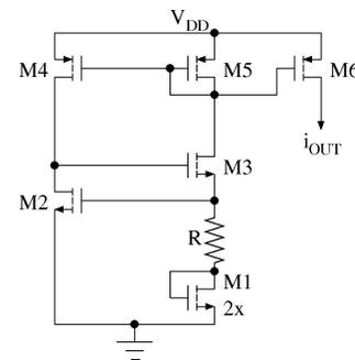
Fig. 11. Sub-threshold current source
