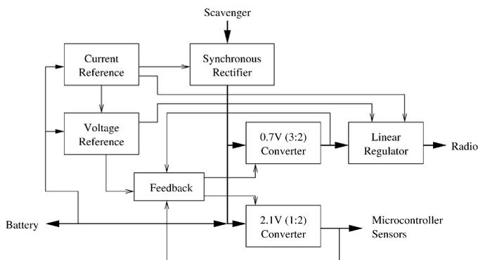
Fig. 3. Block diagram of the converter IC
