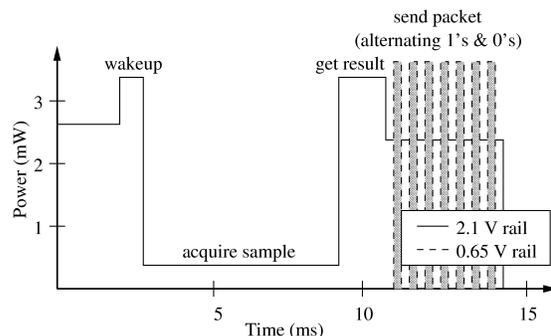
Fig. 1. Measurement and transmission power
