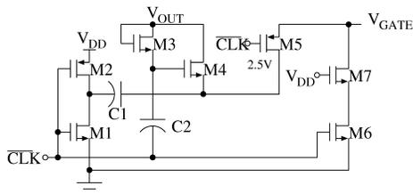
Fig. 5. Capacitor-boost gate drive for the 3:2 converter
