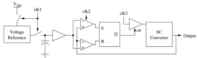
Fig. 7. Diagram of control logic
