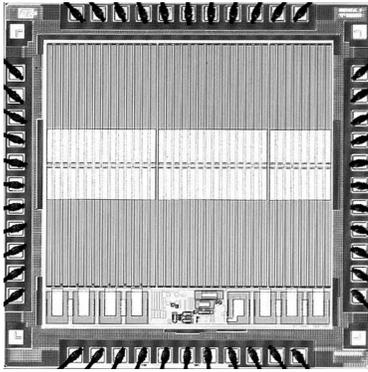
Fig. 8. Photomicrograph of power interface IC
