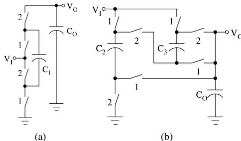
Fig. 3. Switch-level diagram of a) 1:2 converter, b) 3:2 converter
