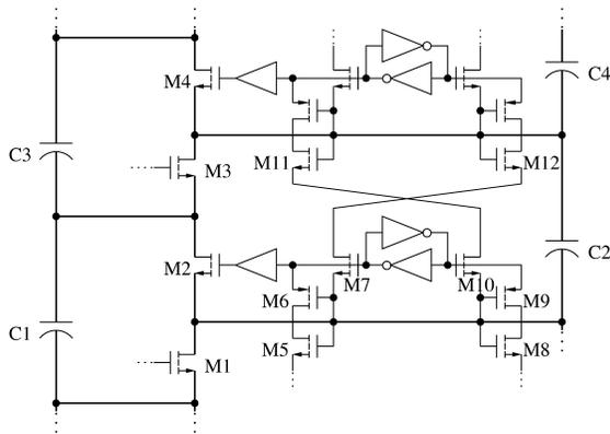
Fig. 4. Cascode level-shift gate drive for the 1:2 ladder converter
