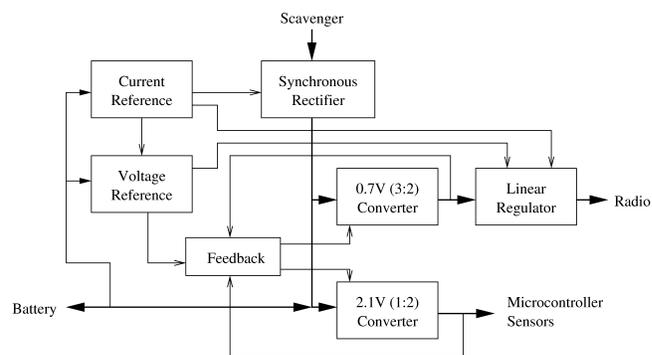
Fig. 2. Block diagram of the converter IC
