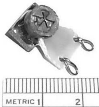
Fig. 9. Partial stator assembly, back iron and permanent magnet not shown.
