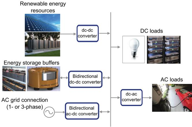
Fig. 1: A prototype nanogrid for power distribution in a smart building.
