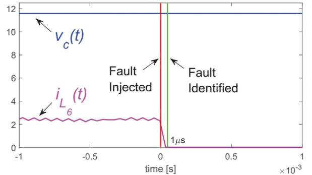
(b) FDI for a sensor fault in  $i_{L6}$ .
