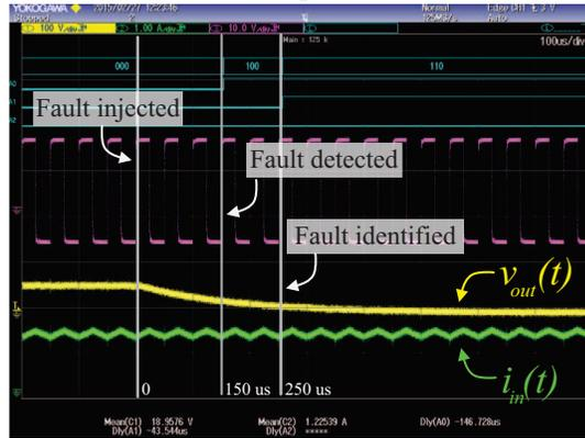
(b) FDI for a sensor fault in  $v_{out}$ .
