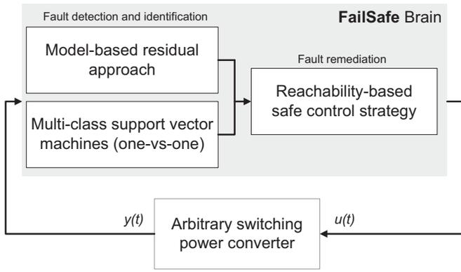
Fig. 2: Overview of FAILSAFE, as applied to an arbitrary switching power converter.
