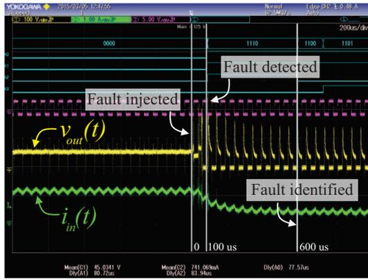
(a) FDI for a component fault in  $C$ .
