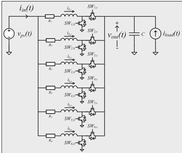
(b) Interleaved boost converter topology.
