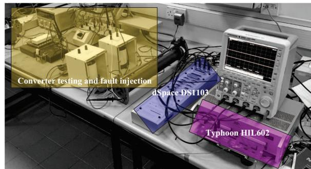
Fig. 4: Nanogrid testbed for validating the FAILSAFE implementation. The converter and FAILSAFE computational hardware are shown.
