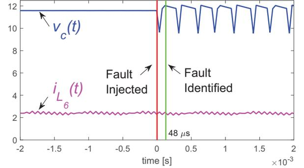
(a) FDI for a component fault in  $C$ .
