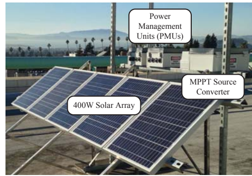
(a) The scaled-down dc microgrid prototype used for experimental validation.
