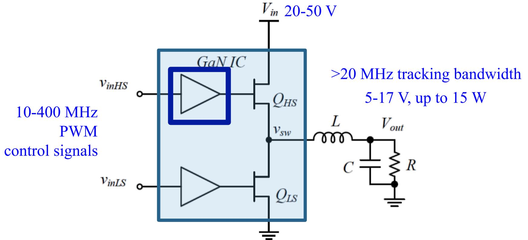
*Key circuit innovation: level-shifting high-side gate driver in GaN-on-SiC process to support very high frequency PWM control*
