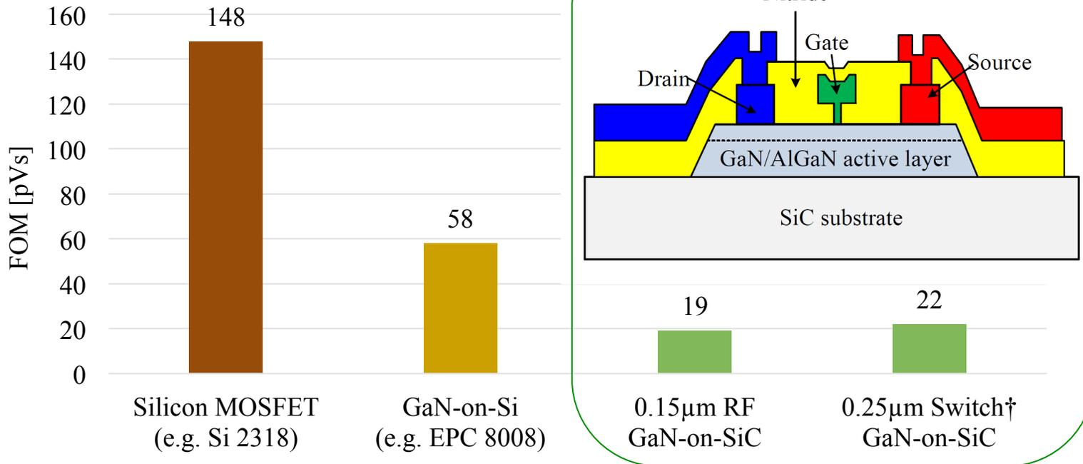
Superior figure of merit allows switched-mode converter circuit design techniques leading to high efficiencies at very high switching frequencies
