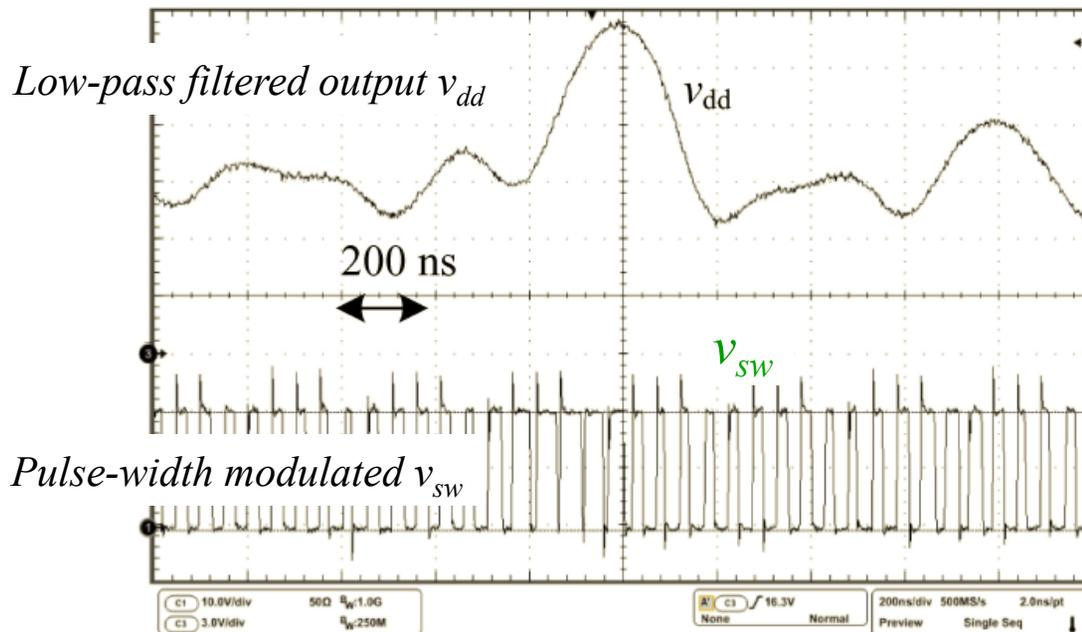
CU CoPEC **Challenge: high-efficiency at high switching frequency**
