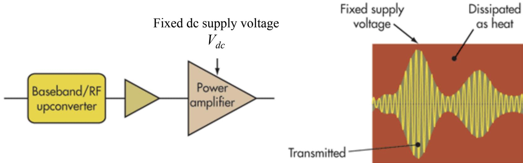
Problem: low efficiency of conventional RF transmitters in mobile, base station, and other wireless infrastructure systems
