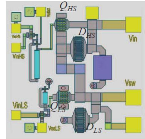
Chip layout:  $2.4 \times 2.3 \text{ mm}$
